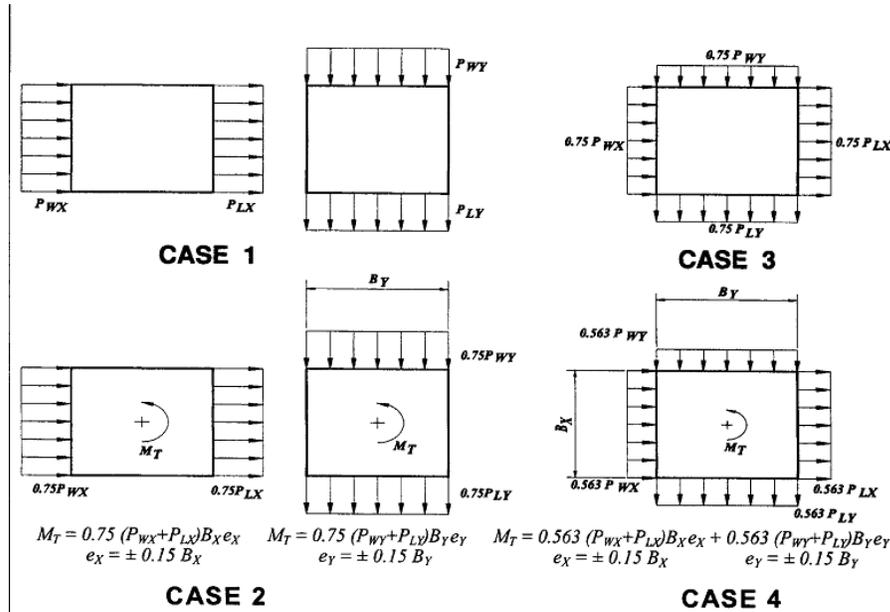
Figure 13: Wind Load Cases from ASCE7-05 Figure 6-9
