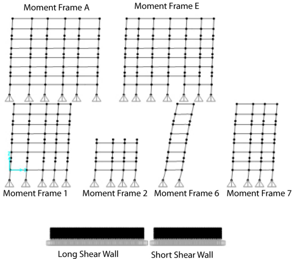
Figure 8: SAP frames under lateral loading
