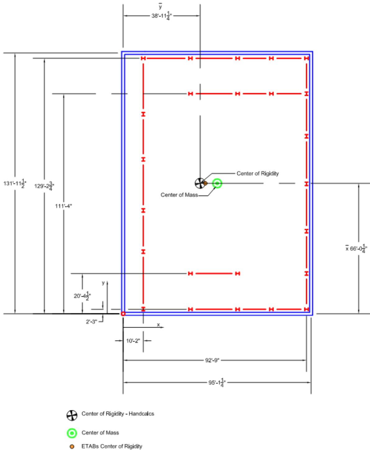
Figure 10: Center of Rigidity for Basement Level
