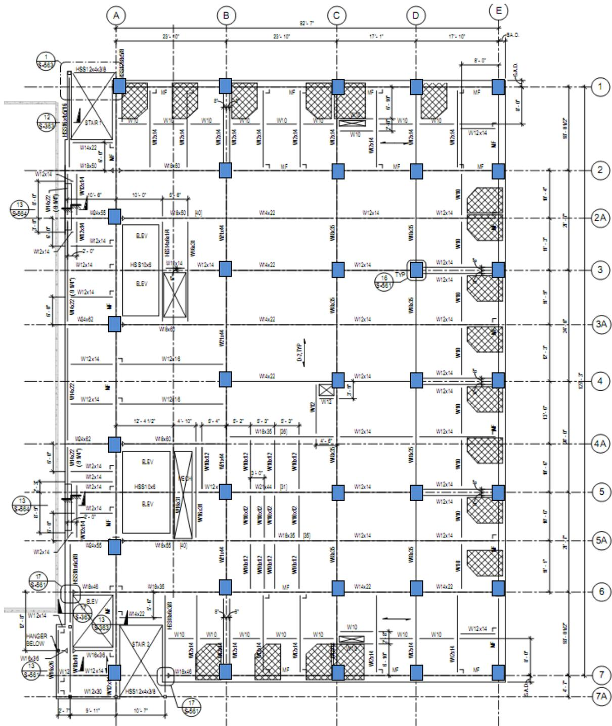
Figure 3: Typical Framing Plan with columns highlighted
