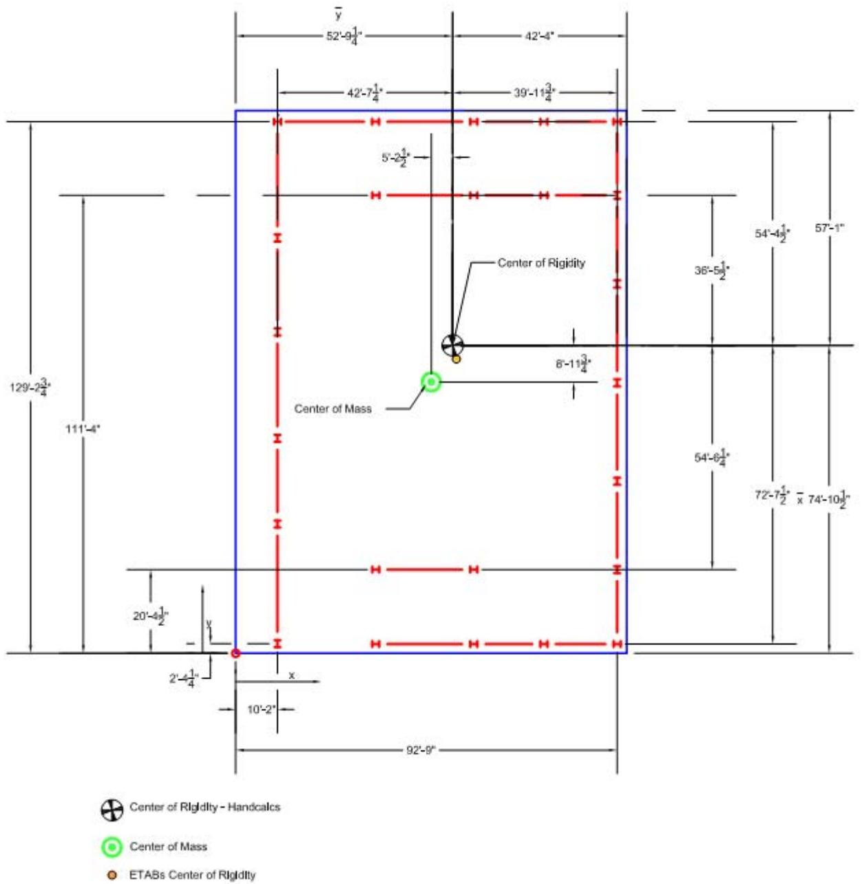
Figure 11: Center of Rigidity for Ground Floor-3rd Floor
