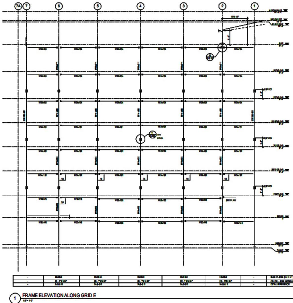
Figure 20: Typical Moment Frame Elevation
