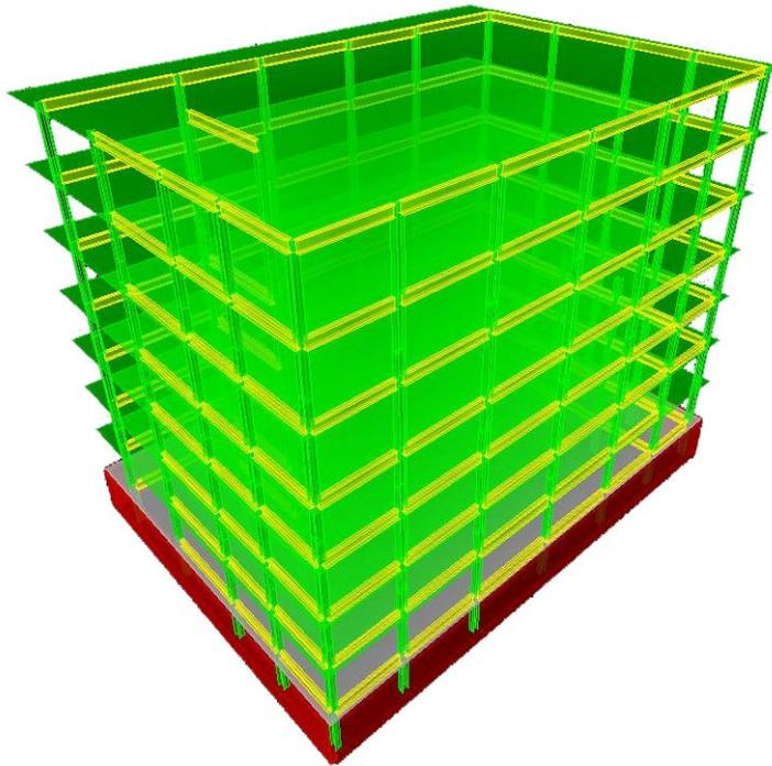
Figure 9: 3D Lateral System Model
